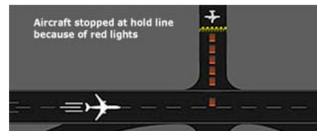
Runway Entrance Lights (RELs) illuminate red when a runway is unsafe to enter or cross due to a high-speed operation on the runway.
