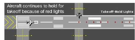
Takeoff Hold Lights (THLs) illuminate Red to indicate an unsafe condition when an aircraft is in position for takeoff and another aircraft or vehicle is on or about to be on the runway in front of it. To be consistent in appearance with Runway Entrance Lights, THLs are placed longitudinally along the runway centreline.
